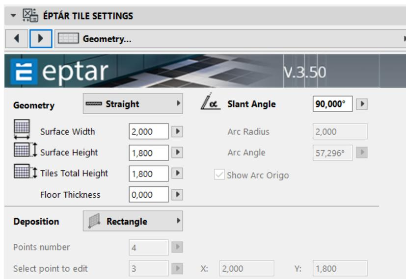
**Geometry:** in add-on mode you can only modify Height offset. For slanted floor surfaces use individual placement (*7 Individual Placement*).
