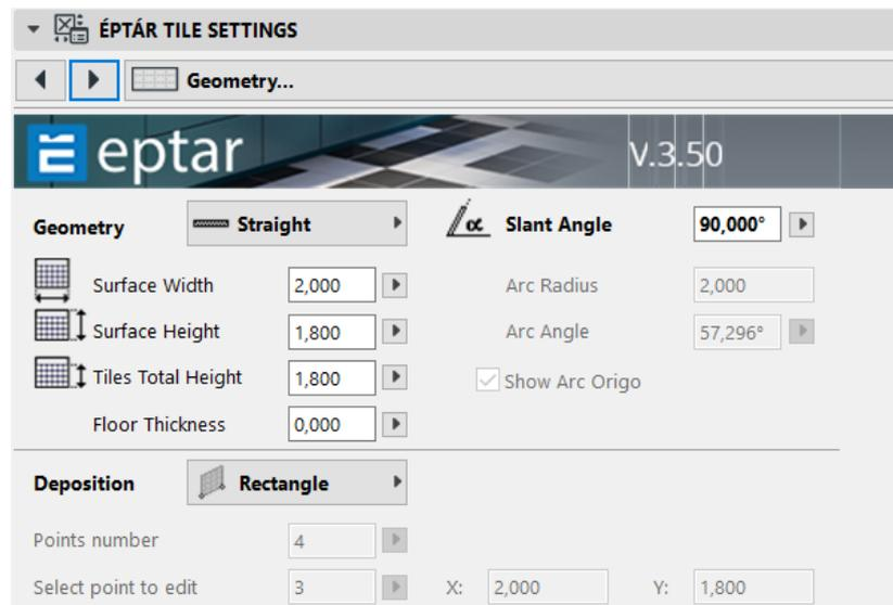
**Geometry:** you can only set the Total Height and Floor Thickness in Add-on mode. If you want to place tiles for slanted, double slanted or curved walls, you will have to use individual placement. (*7 Individual Placement*)
