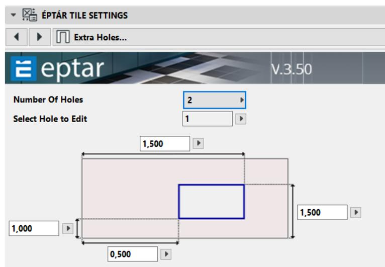
There is no need to tile surfaces behind plumbing fixtures, for example bathtubs. Use extra holes to create untiled patches on your wall. These holes only appear in the tiled surface, they do not affect the wall. To create holes in both the tiles and the wall use Archicad openings.
