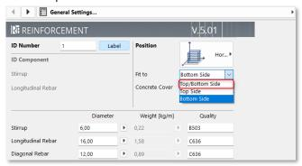
When you have set these parameters, click OK. A window asking "Do you want to assign additional reinforcement to the base AC elements?" will appear. Here it is possible to place additional reinforcements in this element without interrupting the reinforcement process.
