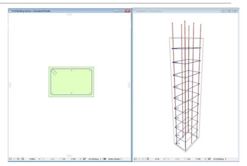
When you are finished with the beam objects rebar structure, select all the rebar, stirrup abd concrete elements in the crowning and make sure that the **"Use for Listing**" parameter is selected.
