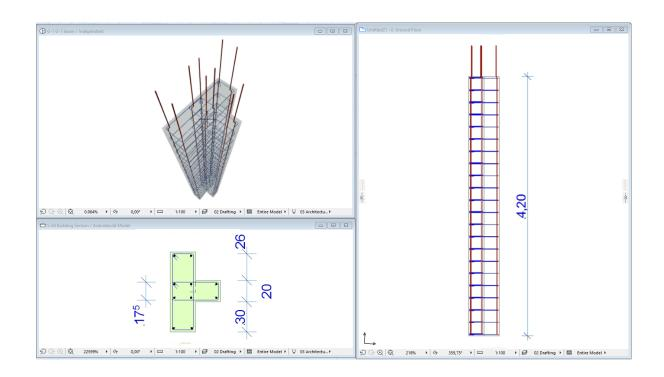
When you are ready with the column objects rebar structure, select all the rebar, stirrup, and concrete elements in the Column and make sure, the "Use for Listing" parameter is selected.
