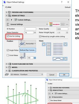
There is a **"for Listing**" switch in every element. Sometimes, some elements are only placed for a complex element's creation in the model space, or maybe an explanation, and bars as outstretched views. In these cases, these bars can be left out from the optimization and listing. This switch is basically switched on so every element will be listed. When switching off, be careful so that you don't miss out elements which you want to show in the list from the listing.
