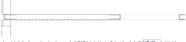
To place labels for the section drawing use ArchiCAD label objects. Select the **"Label**" (<u>**-**At Label</u>) object from the toolbar. Open the **"Label Settings**" dialog and select the **"rf\_label**" type for objects. Click the **"**OK" button.
