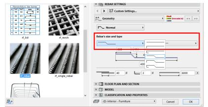
If you need more rebars in the crowning, go back to the Floor Plan view and multiply your rebar object on the Floor Plan to the right positions.
