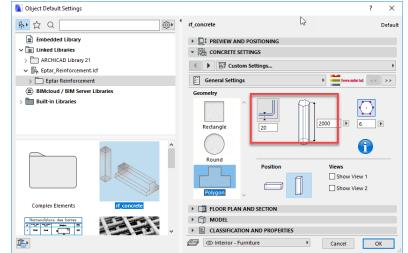
Normally, the columns and beams have a constant section along the full length, so one concrete object is enough to define the external shape of the complex element. If you need more complex shapes, you can use more concrete elements to define the final shape.
