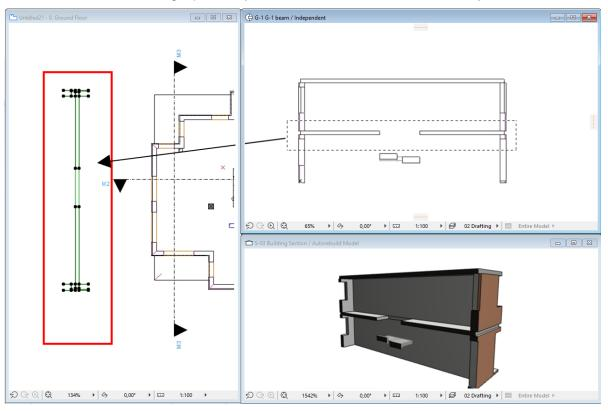
Select one of the rebar objects which crosses the section line on the Floor Plan. Open the **"Object Settings**" dialog and click the side view icon on the **"General Settings**" tab page.
