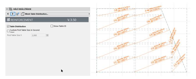
If, due to the shape of the structure, it is simpler or more economical not to distribute the mesh boards at the same time, then its surface can be planned to be laid in several directions. This is a more flexible board layout design
