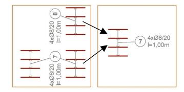
After the automatic calculation and ID check you have to define the position of the cutting list on the Floor Plan. If you have a cutting list on the Floor Plan already, the software does not place a new one but refreshes the existing one.
