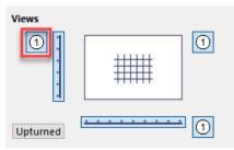
You can set the display of labels on the "Labels" page. If you have turned the "Show Label" switch on, the mesh will be labeled according to the label type you chose. Content of the label could be overwritten on this page: you can decide whether you want to see the ID, measures, diameter of the rebars on the floorplan. You can also choose the shape of the marker and add a custom text to your label.
