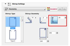
Select the stirrup section form and set up the parameters on the **"Geometry**" tab page.
