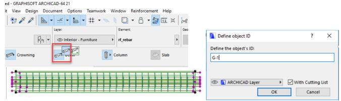
this name as well for the components (rebars and stirrups) of this column. In the dialog, you can see a check box with a name **"With List**". If you click this check box (default), you can place an individual rebar table about this construction on the Floor Plan (useful for detail drawings). Click the "OK" button.
