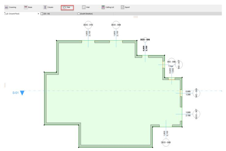
Select the ArchiCAD slab or wall objects to fill out with rebar or mesh elements. Use **"Floating palette / Slab or Wall**" command. Select the rebar or mesh object in the dialog box and set up the necessary parameters as we defined in the earlier chapter. Click the "OK" button. ArchiCAD automatically places the rebar or mesh elements into the polygon shape slab or wall with the parameters already defined.
