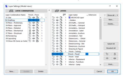
Open "**Document / Layers / Layer Settings**" menu. Among the layers, create (top right button) new layers for the reinforcement plan. We recommend the creation of the following layers:
