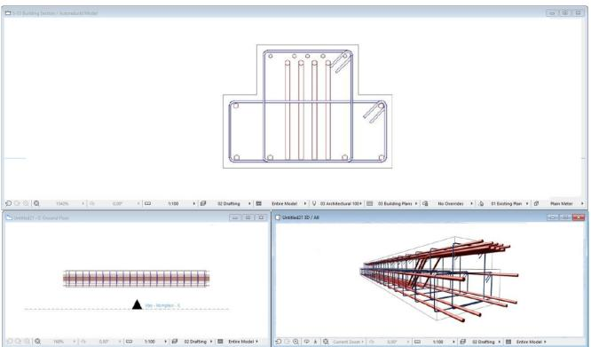
When you are finished with the beam objects rebar structure, select all the rebar, stirrup and concrete elements in the beam and make sure that the **"Use for Listing**" parameter is selected.
