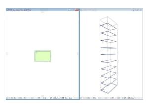
Select the **"rf\_rebar**" object from the library. On the User Interface select the **"Vertical**" placement option and switch on the **"Only one rebar**" check box. Set up the **"Straight**" style of the endings in the **"Geometry**" tab page. Click the **"OK**" button. Place the rebar object inside the stirrup contour. Click on the Section window and move the rebar on the right position with the right length.
