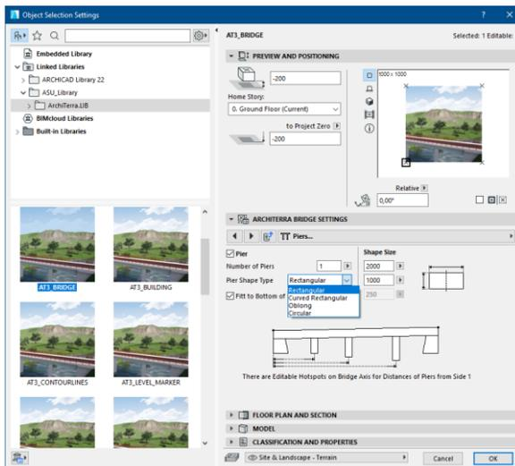
On the 3<sup>rd</sup> tab of the Bridge settings window you can apply Piers, if the Bridge is too long. The size, the shape of the Pier (Rectangular, Curved rectangular, Oblong, and Circular), and the amount of them can be set. You can also decide how the pier connected to the deck of the bridge: fit to bottom of bridge or not.
