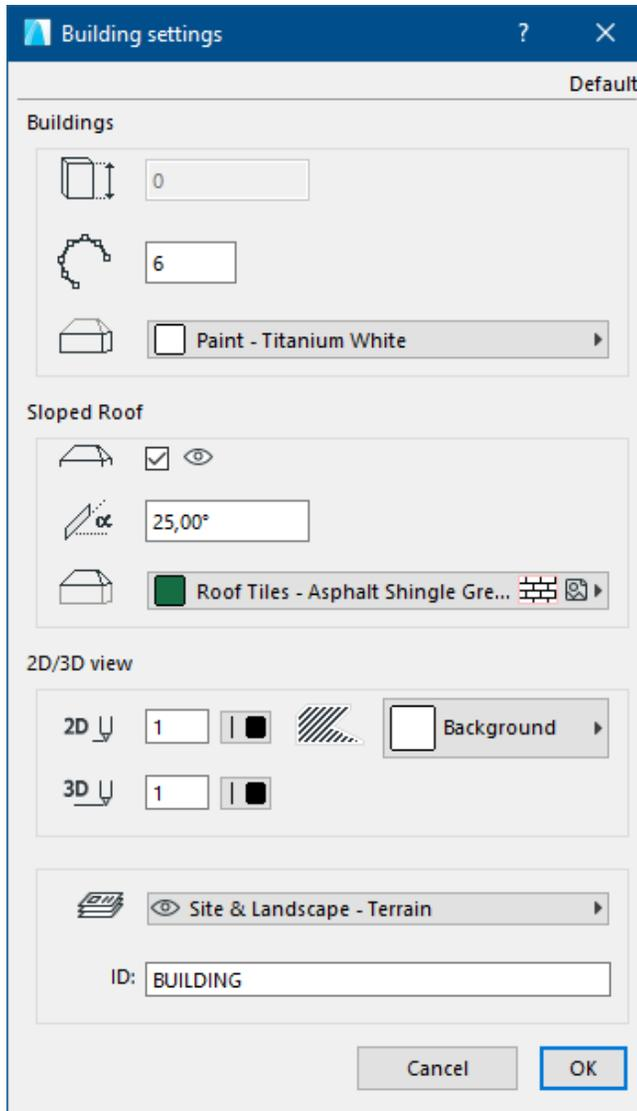
The first field defines the altitude of the eaves of the building to be created as the relative altitude (the height of the building, in other words, the distance from its lowest point to the line of the eaves).
