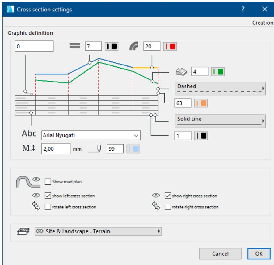
The numerical field at the top left enables to set the reference altitudes (within the limits of the interval available). The user can use this field, for example, to align the various longitudinal sections and make them congruent.
