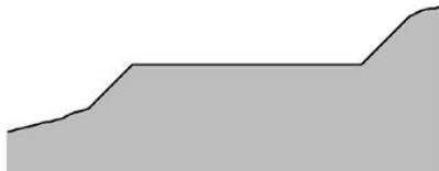
Considering the terrain as a solid and thinking in terms of Boolean operations, the solution to model the terrain in such a way as to obtain the required plateau would be as follows.
