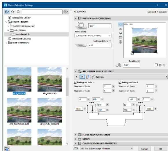
On the 4<sup>th</sup> tab of the Bridge settings the Railing can be set on both sides with size, position parameters. You can set the the number of Posts and Rods separately, set the size of them.
