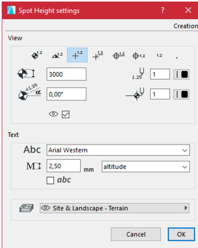
In the View section, it can be configured the appearance of the marker by choosing the style and defining the dimensions, angle and pen used to draw it. In the Text section, it can be chosen the font, size of character and possible use of italics for the string of information to be displayed.
