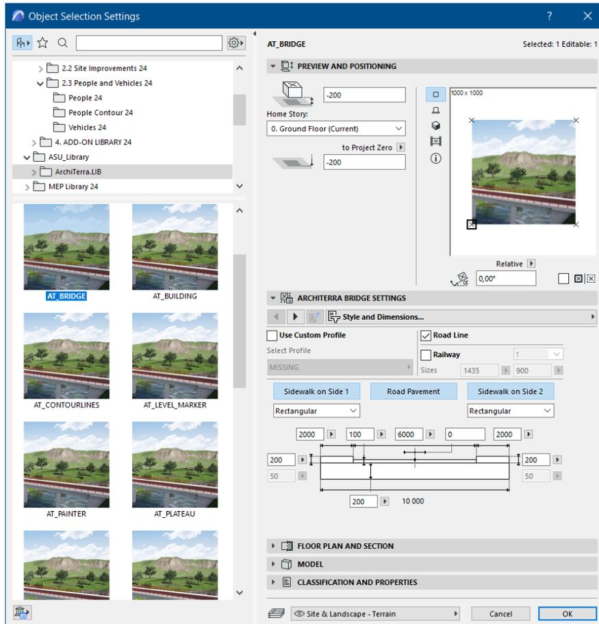
On the first tab you can switch on/off the road line and set the custom profile for the bridge deck, even for Railway bridge. The default profile is a simple slab, no in this case you can define the sidewalk on both side and the pavement.
