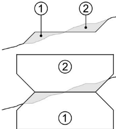
Solid number 2 is the solid which “excavates” and which will therefore be used in the Boolean subtraction. Solid number 1 is the solid which “fills” and which will therefore be used in the Boolean addition.
