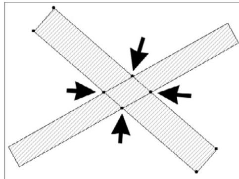
At the junction, each of the two roads will now have editable nodes that can be used to adjust their shape.
