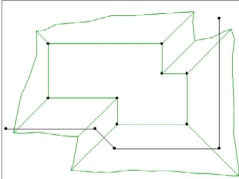
Select the element to be limited (in our example, a plateau) and the polyline representing the obstacle and then click on the Retaining Wall icon in the ArchiTerraPlus toolbox.
