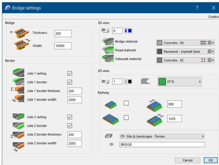
After setting of required parameters click on OK and the program will place a bridge element on the predefined line between two road ends on the level of roads. After the bridge is placed, you can set many other parameters and functions in the ARCHICAD Object Settings window. Select the bridge element and open a setting window:
