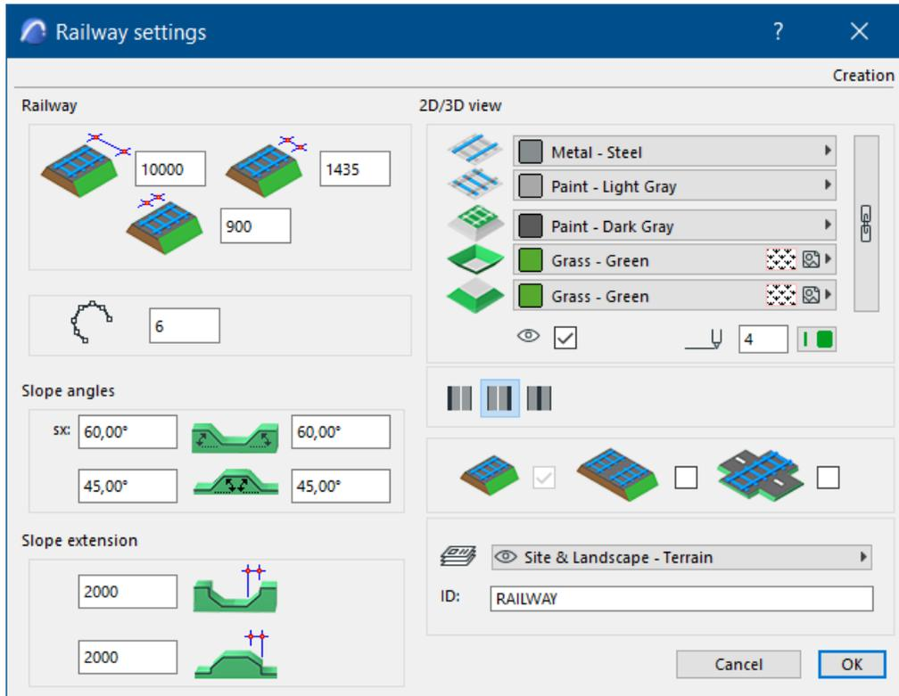
The first value in the Railway section indicates the width of the railway. Use a polyline to create Railway with a constant width.
