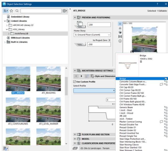
When you select a Custom profile the width of the bridge, the sidewalk and the pavement will be the size what you defined in the Profile Manager. If you would like to change these sizes you should edit the profile in the Profile Manager and save it.
