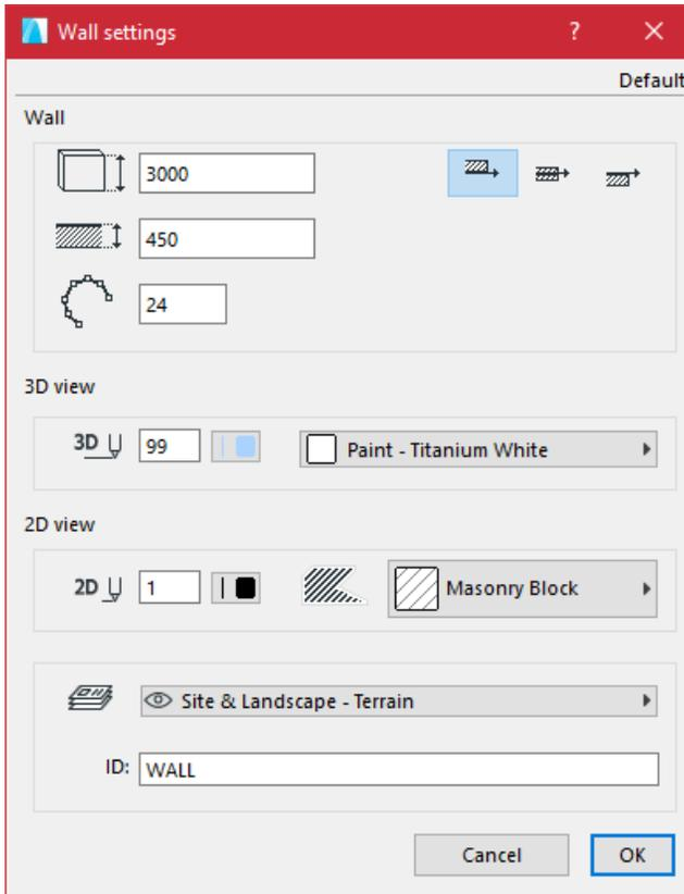
The user can define the height of the wall (constant along the full length) and its thickness, while the three buttons on the right define the position of the wall with respect to its reference line.
