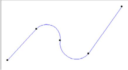
Using the *ArchiTerraPlus Polyline tool*, draw a polyline to create the centre line of the road to be created.
