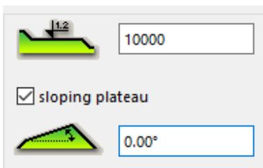
When the check-box is activated, the field below is enabled and it can be defined the slope of the plane. All other fields have the same function as described previously, configure as required and click on the OK button.
