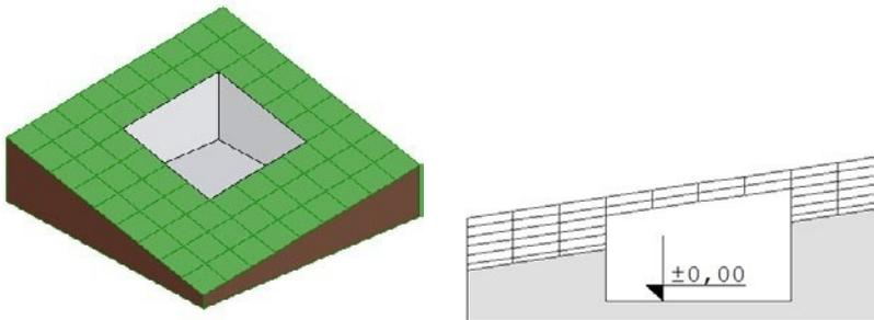
Using Solid Elements Operations, the volume of the slab is subtracted from the mesh: As can be seen in the cross section, the altitude of the mesh corresponding to the plateau obtained by subtracting the volume of the mesh is 0.00 meters.
