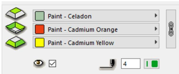
In the 2D/3D View section, users can configure whether the perimeter of the excavation will be displayed in the map view (by activating the relative check-box on the left) and the pens used to represent the edge of the excavation in the map and 3D views.
