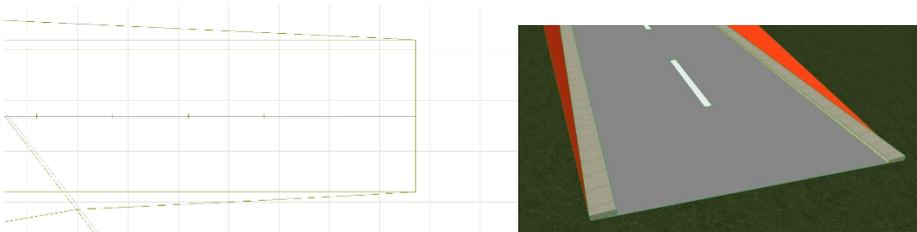
Creating a road using an ARCHICAD fill as described above, by using a polyline the user will obtain a “regular” shaped road only (although by dragging the editable nodes subsequently, it can modify the morphology).
