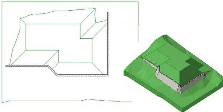
The following diagram shows the meaning of the values in the Wall section of the Retaining Wall settings dialog box:
