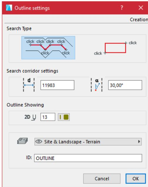
The drawing option using the two buttons on the dialog box can be chosen to define the type of outline: polygon or rectangle.
