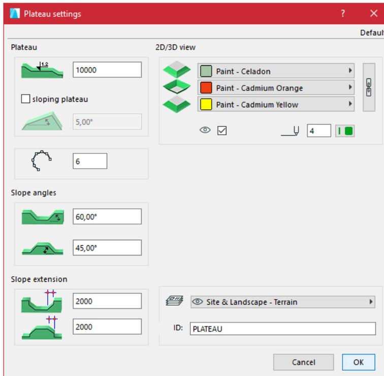
In the section at the top left labelled Plateau, it can be defined the height and type of the plateau, given that users can create either horizontal or sloped plateaux. In this example the sloped plane option is disabled and a plateau with a horizontal plane will therefore be created. How to create a plateau with sloped plane will be described in detail in the following paragraph.
