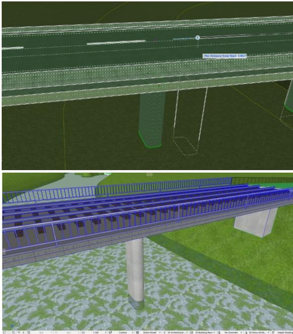
The position of the Piers is modifiable graphically with hotspots in 2D and 3D.
