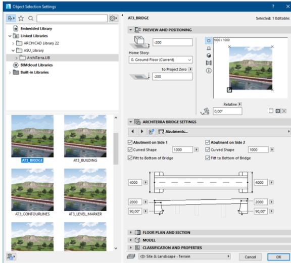
On the next TAB of the Bridge settings window you are able to switch the Abutment on both ends of the Bridge. The size, the shape of the abutment (curved or rectangular), and the Inclined Angle of it can be set. You can also decide how the abutment connected to the deck of the bridge: fit to bottom of bridge or not.
