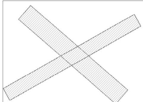
Draw two fills to represent the roads and in each of the two fills, add four nodes at the junction with the other fill/road:
