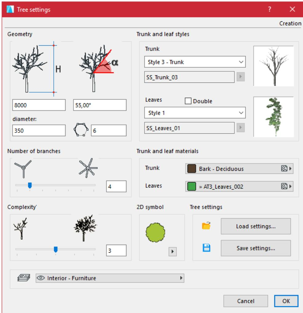
In the Geometry section it can be defined the total altitude of the tree, the angle of the branches with respect to an imaginary horizontal line (the value can be negative to generate conifers), the diameter of the trunk and the resolution used.
