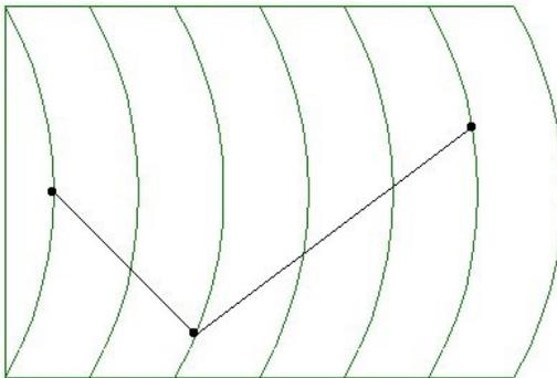
As explained above, when this polyline is transformed into an ArchiTerraPlus wall, ArchiTerraPlus will use the three nodes to acquire information on the altitudes of the terrain and then construct the resulting wall. Then select the polyline and the terrain/mesh and click on the Wall tool in the ArchiTerraPlus toolbox to display the Wall settings dialog box, confirming the default configuration.
