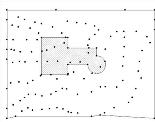
To create a plateau, first draw the perimeter of the area to be levelled using the fill tool and then select the fill to be processed.
