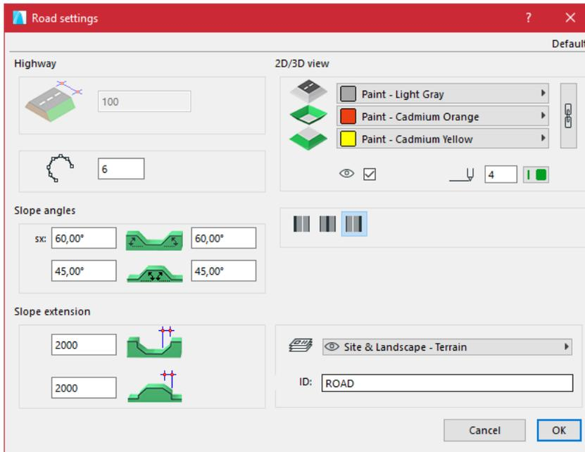
The first value in the Road section indicates the width of the carriageway. Use a polyline to create “regular” roads with a constant width (although by dragging the edge nodes, it can easily modify the shape afterwards).
