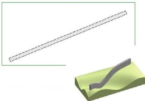
If you move the cursor to the two sides of the polyline, the arrow changes direction, indicating the side on which the Retaining Wall will be constructed. Click on the required side and ArchiTerraPlus immediately generates the element requested.
