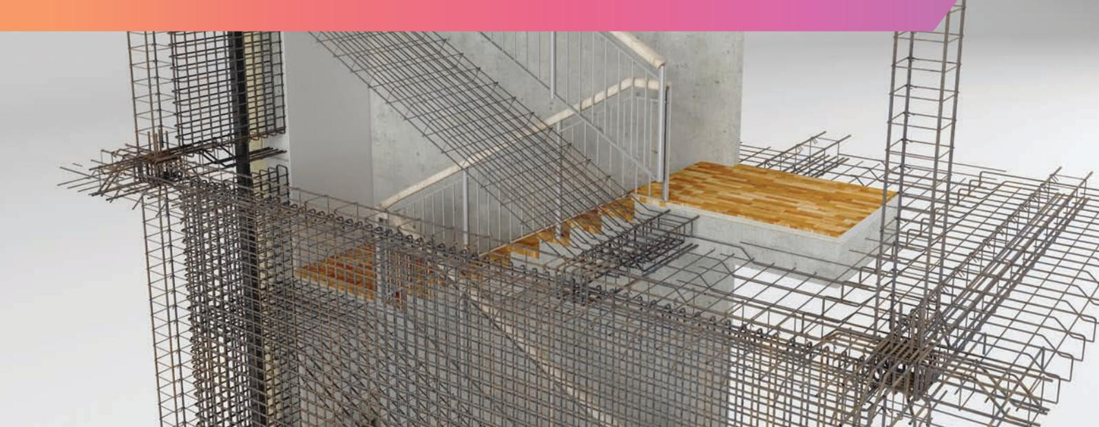
This solution helps designers to draw documents and lists the necessary reinforcement for their buildings in ArchiCAD. The application provides tools to define all 2D drawings as well as complete 3D models.
