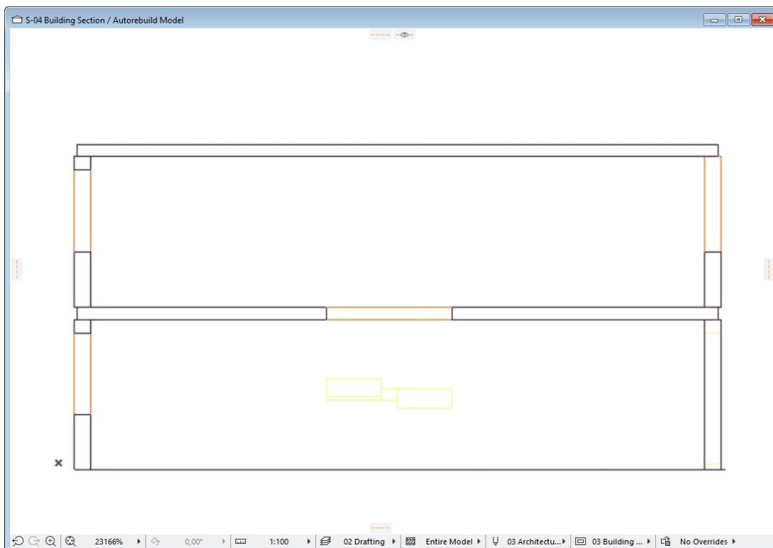
Set up the „**M-1**” Section as a „**Trace**” view in Section „**V-1**”. Open the „**M-1**” section view and set up the „**Layer Sets**” to show the slabs in the model in „**Wireframe**” mode. If you followed these steps, the rebar objects will be visible in the „**M-1**” section.
