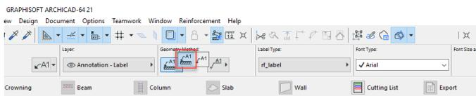
On the working area select the „**Label connection to objects**” placement method. In this case, the settings of the label, such as text and shapes, will be set directly on the Reinforcement object interface, in the Label tab. By choosing the „**Independent**” placement method, the changes are set in the Label Default settings.
