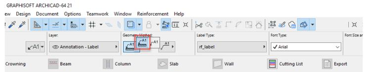
This Label will be connected to the rebar objects until you delete it, the label will be update at all parameter changes and the label will move with the object together.
